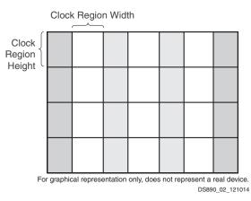
Figure 2: Column-Based FPGA Divided into Clock Regions
