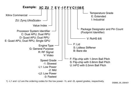
Figure 5: Zynq UltraScale+ MPSoC and RFSoC Ordering Information
