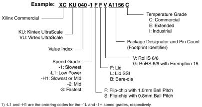
L1 and -H1 are the ordering codes for the -1L and -1H speed grades, respectively.
